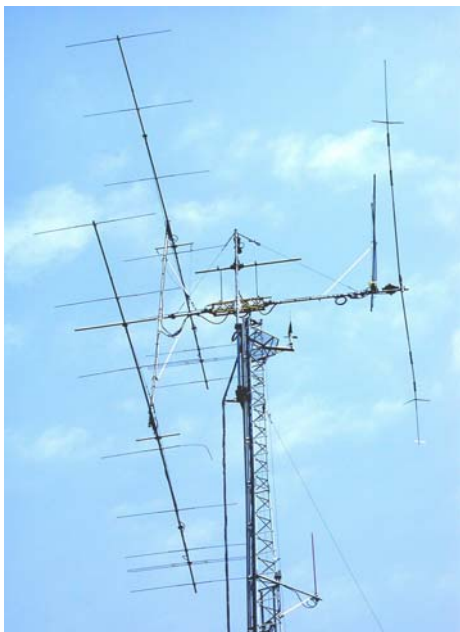
Figure 5: JE1BMJ's 10.7m boom, eight-element yagis stacked 7.7 m apart with an elevation rotation mechanism.
